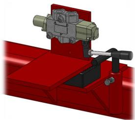
Figure 3.2.3-Hydraulic limit switch
