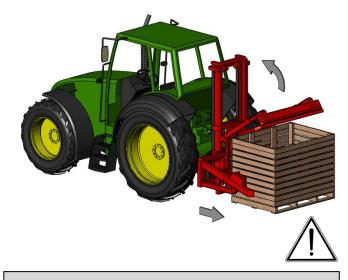
Raise the upper clamp using the clamping cylinder before picking up the box with the box rotator. Distribute the load as evenly as possible over the forks.
