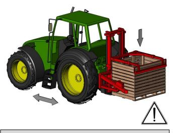
Keep the load as low as possible during transportation to maximise the stability of the lifting vehicle. Boxes must always be clamped during transportation.
